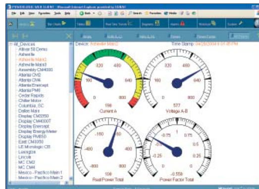
Meters with color bands act as maintenance "grease marks" for normal range indicators allowing visual inspection to view amps, volts, power and power factor at a glance.
